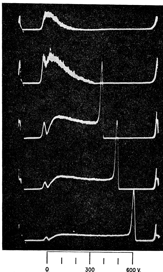
FIG. 7. Oscilloscope display of the energy distribution of Ar^{++} from an argon discharge. Discharge pressure = 0.5 Torr; discharge voltages (top to bottom) 300, 350, 400, 500, and 600 V; vertical sensitivity 0.05, 0.5, 1, and 2 V/cm. The discrimination at low ion energies causes the unusual shape at the left.
